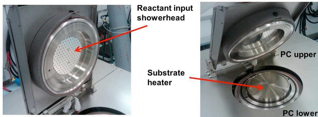
**Fig 3:** Reactant input showerhead and upper/lower chamber
