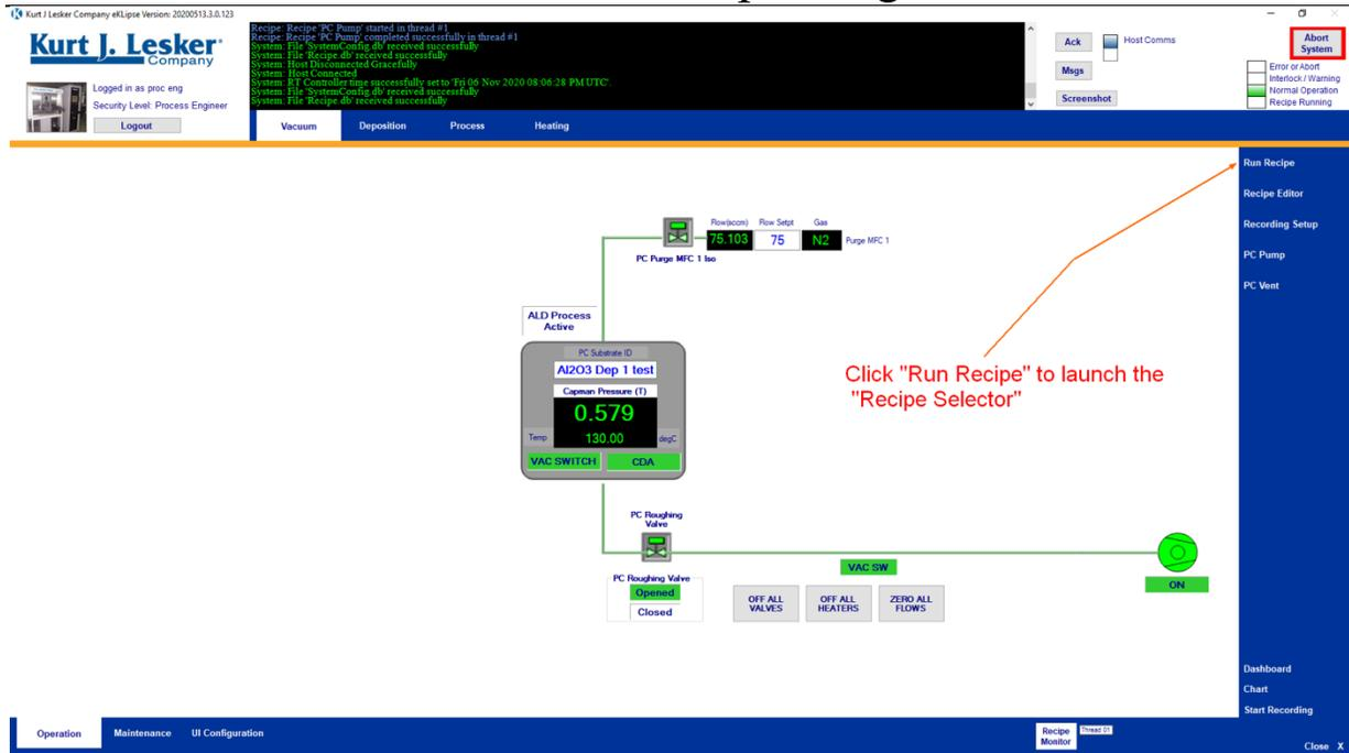
Fig 4: Vacuum screen –Run Recipe on the top right
