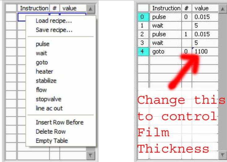
Fig 1. Loading of recipes; only select the Load Recipe option; only edit **goto** line.
