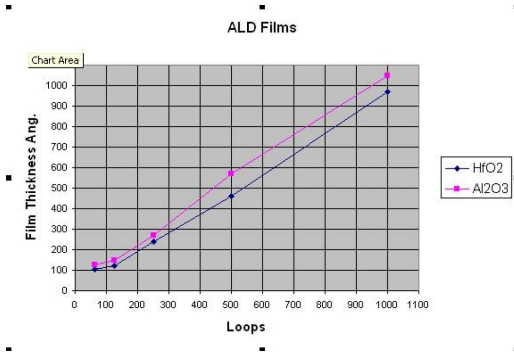
Fig. 5: ALD film thickness for Al<sub>2</sub>O<sub>3</sub> and HfO<sub>2</sub> films.
