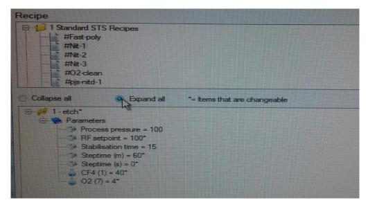
7.3.3 Modify the parameters as needed. To modify a parameter, double click on the parameter and then enter the new value. "step time" refers to the etch time. There
