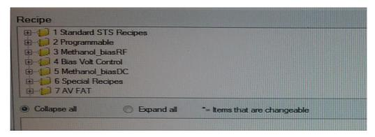
7.3.2 A recipe selection window will pop up allowing you to select the desired etch recipe from a list. Click on the "+" to expand the folder that contains the desired recipe, i.e. Standard STS recipes folder, Programmable folder, etc. In the selected folder, highlight the desired etch recipe, then move the cursor below and click on "Expand all".
