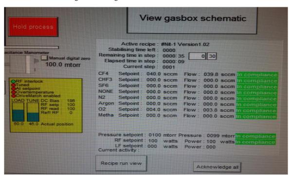
Note that if you want to abort the process before the timer goes to "0", you can press the "ABORT" button on the left side of the screen. After a short time, a message will pop up that reads "PROCESS FAILED". Click "OK" to acknowledge message. An event monitor on the lower right side indicates the status of any ongoing process at any time. In this case, it will indicate that the process error is due to the process being aborted.
