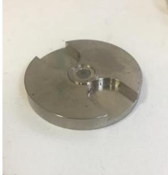
magnetic holder. **DO NOT** put sticky tape between the puck and magnetic holder! Mount the magnetic holder on the sample block in the center. Wafers can be set on top of the sample holder and scanned with/without vacuum.
