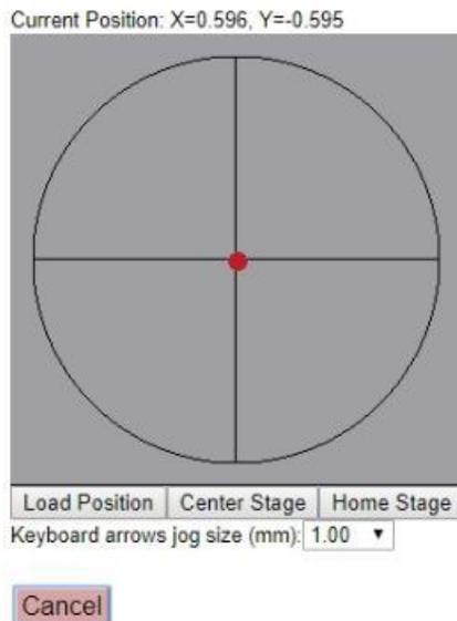
Fig 1. This is the display that is shown when the stage movement control is working. Just click anywhere on the image and the stage will move to that position.
