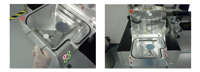
i. Load the dummy wafer onto the robot arm, taking extra care to gently align the wafer's major flat up against the two pins that are farthest from the chamber. Then gently align the left side of the wafer up against the left-most pin. When loaded properly, the dummy wafer should be oriented like the image below:
