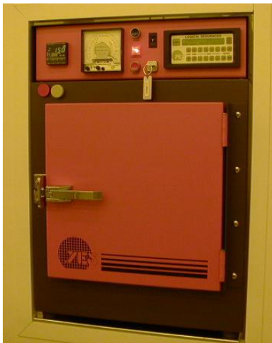
Figure 1 The image reversal oven in Keller Hall-Bay 2.
