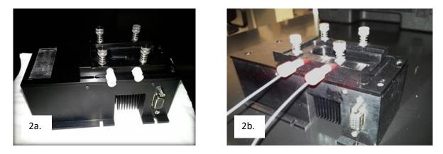
Figure 2. Laser module with flow cell and Luer plumbing attached.Fig 2a. Luer syringe fittingsFig 2b. Luer fitting plus 1/16" tubing for syringe pump.
