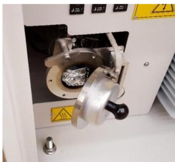
**Figure 7** Load the dimer filled boat into the vaporizer with the dimer filled side closest to the door.
