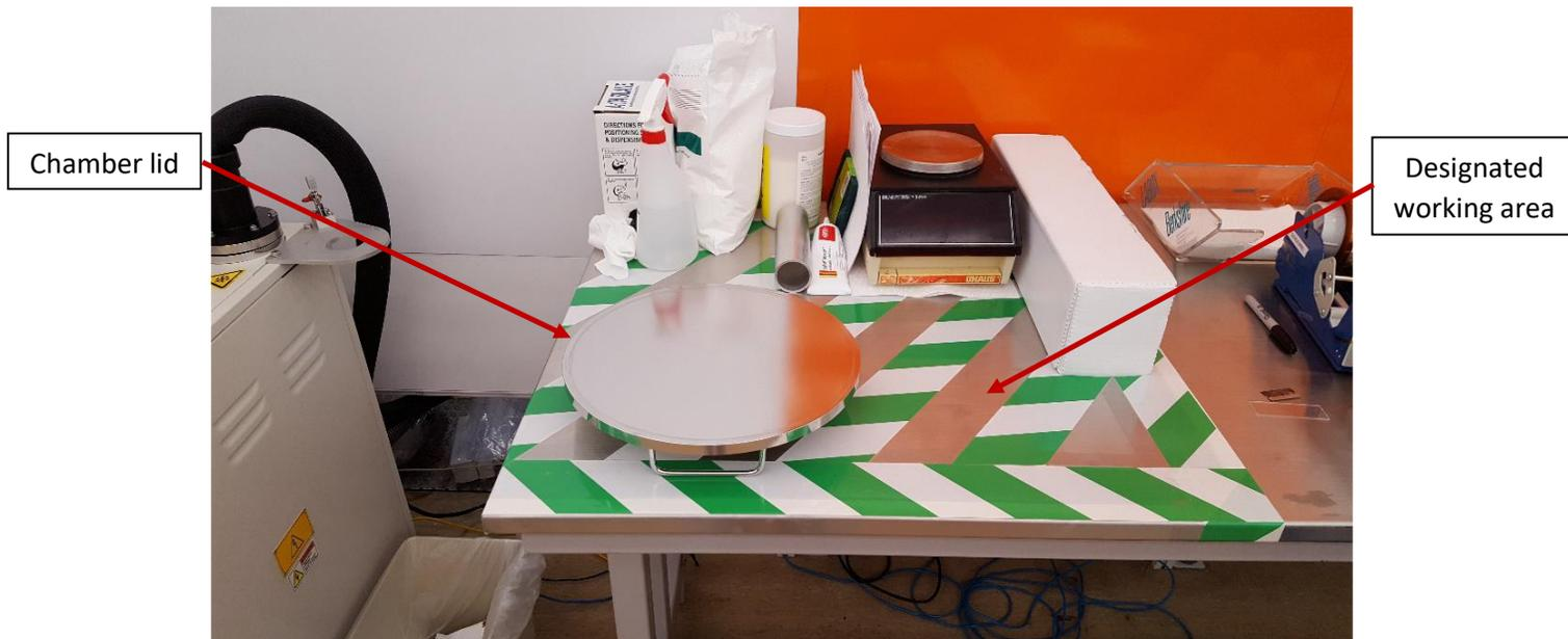
**Figure 4** A designated working area is marked with green and white tape. Take care to place the chamber lid handle side down to prevent scratches to the sealing surface.
