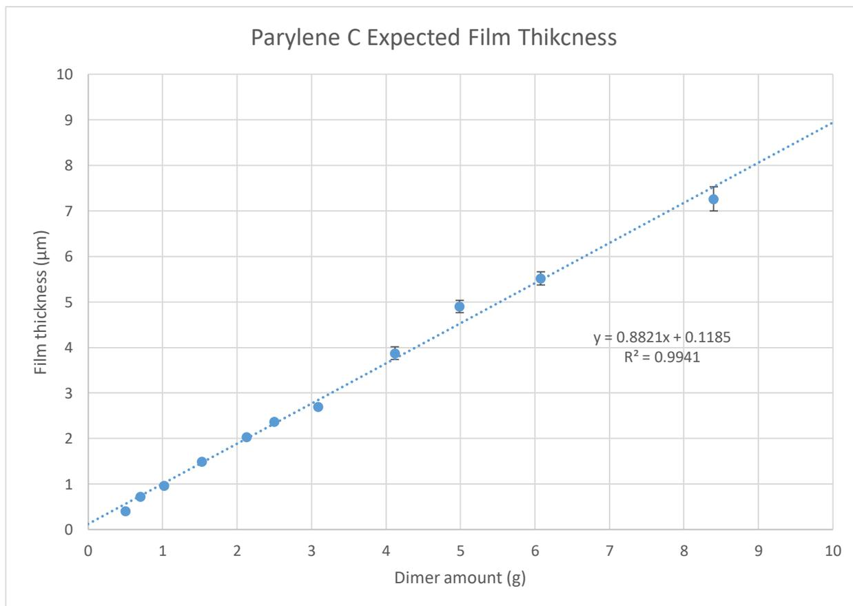
**\*\*This tool was characterized using a flat silicon wafer on the edge of the rotating platform. Measurements were taken using a profilometer.**
