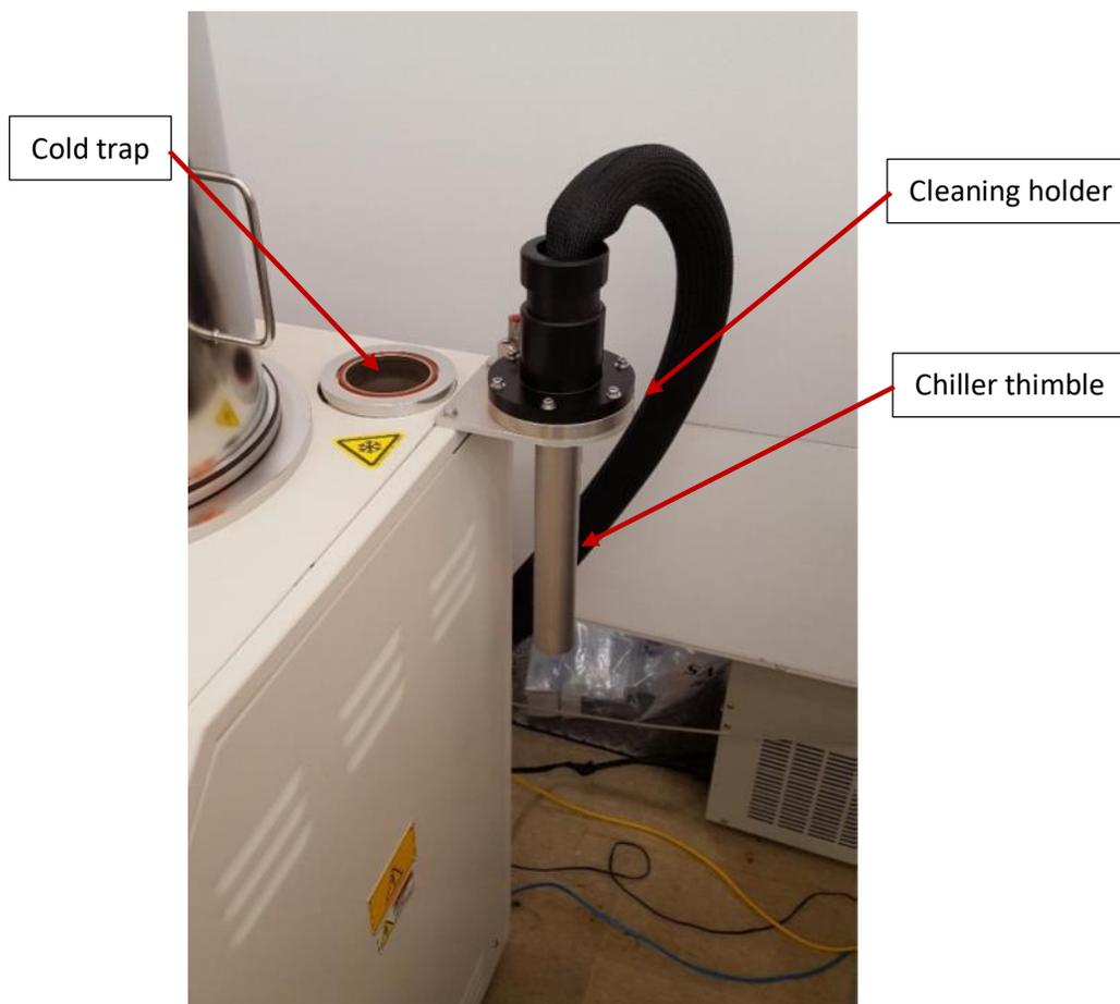
**Figure 8** A cleaning holder is provided for the chiller thimble. After turning off the chiller wait 5 minutes before moving it to the cleaning holder. After waiting an additional 10 minutes, or until the water crystals start to melt, clean the Parylene off of the chiller thimble.
