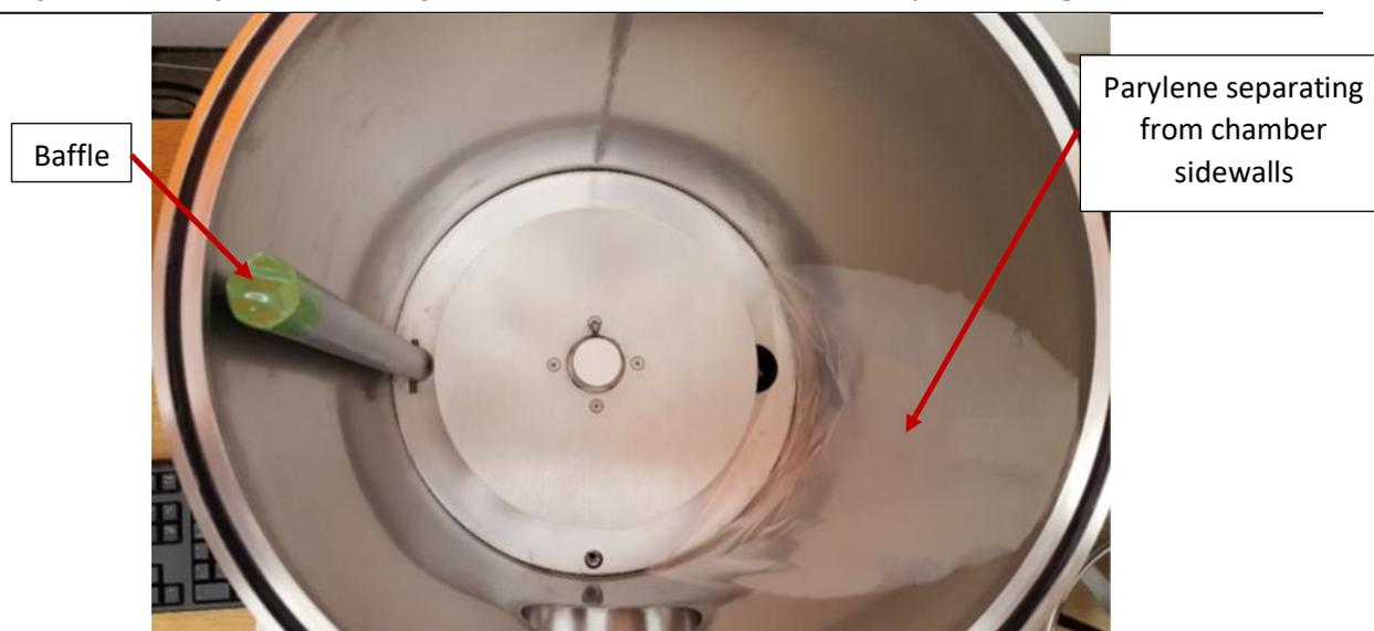
**Figure 5** *If Parylene is separating from the chamber sidewalls, do not continue. Cleaning is needed and should be reported to MNC staff via Badger*
