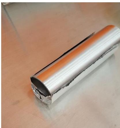
**Figure 2** Use the boat former to mold the aluminum foil. The boat should not be longer than the boat form.
