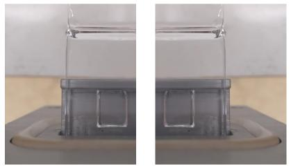
Verify that the quartz tray is well centered on the aluminum support lip by inspecting the left and right sides of the support lip (as shown above). This ensures that the tray is not positioned too far to the left or right, which will help to prevent the tray from hitting the door flange or the inner walls of the oven.
