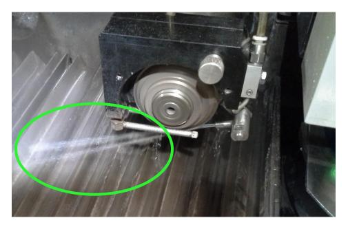
If the stream doesn't appear to split as shown in the image above then the water nozzle position will need to be adjusted. If this is needed, then you will need to grab the water nozzle at the following location (see image below).
