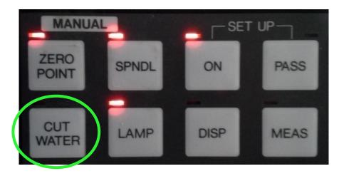
Once the cut water is on, move your Styrofoam splash shield as needed in order to keep as much water in the machine as you can. If the water nozzle located on the right side of the dicing blade is in the proper position, you should see the water stream split into two streams (see image on next page).
