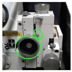
Use the fine focus knob to make any other focus adjustments to optimize the focus on your feature of interest. To do this, unlock the **fine focus knob** by turning the **lock-lever** counter-clockwise until it is loose. Then turn the **fine focus knob** to finish focusing your sample. Re-lock the **fine focus knob** by turning the **lock-lever** clockwise until it is lightly snug. See image below for fine focus knob and lock-lever locations.
