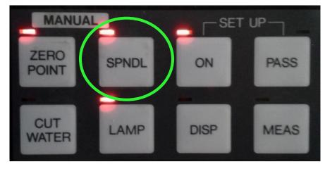
Once the spindle is off you should hear a loud click. This is a safety solenoid that will secure the left safety cover during dicing. Now that the safety solenoid is open and unlocked, close the left safety cover all the way by lifting up the black handle, pulling toward you, and then pushing the black handle down firmly.
