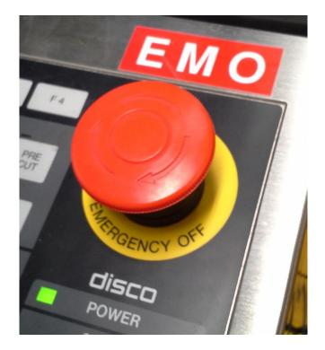
Ensure that your hands are free and clear from any moving parts in the <u>chuck or</u> <u>spindle area</u> and exercise great caution whenever the spindle is rotating and/or whenever the safety covers are open.
