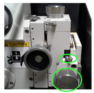
Most users will want the hairlines centered vertically on the monitor so that they coincide with the horizontal crosshair line in the microscope eyepiece.
