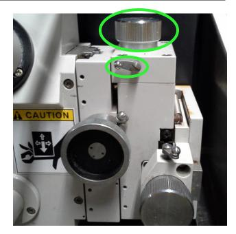
**k.** <u>Sample Alignment</u>: Look in the microscope eyepiece and you should see a set of perpendicular crosshair lines. The sample or feature of interest will have to be aligned to the horizontal crosshair line. You should also see one or three horizontal hairlines on the computer monitor.
