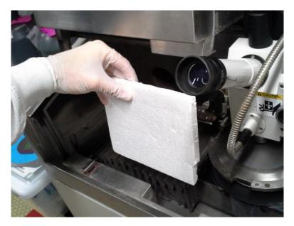
While holding up the piece of Styrofoam with your left hand, use your right hand to turn on the cut water by pressing the **Cut Water** button (see image below).
