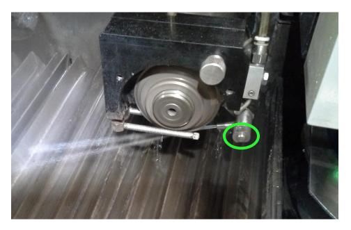
With your right hand, CAREFULLY grab the water nozzle by pinching it with your thumb and index finger and then pull or push the nozzle gently as needed. You may have to rotate the nozzle as well if it's not hitting the blade at the proper angle. Adjust the nozzle position as needed to satisfy both conditions as listed on page 16. Once this is set properly, press the **Cut Water** button to turn off the cut water.
