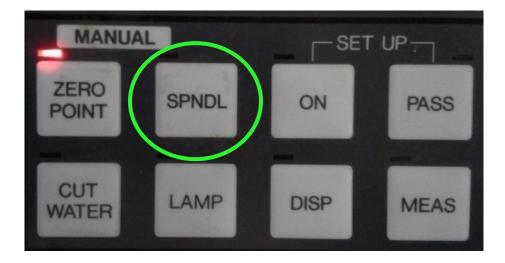
Turn **ON** the spindle rotation by pressing the **SPNDL** button (see image below):
