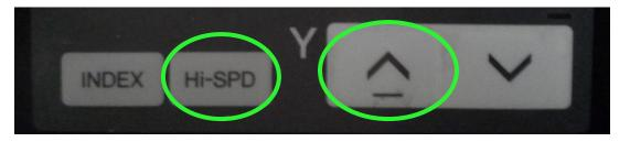
As you hold both of these buttons down you should notice the spindle and microscope move backward. Once the spindle is all the way back to the Y-axis upper limit you will hear an alarm beep. You will also notice an alarm displayed on the bottom left of the computer monitor which says: "Y: REAR LIMIT END". This is normal. Press the ESC button to acknowledge and silence the alarm.
