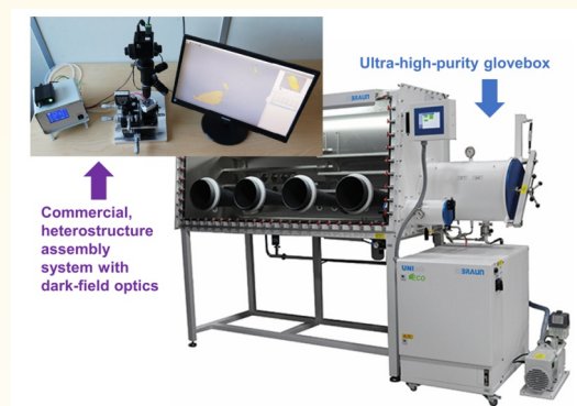
Image showing the primary components of the ultra-high-purity heterostructure assembly system.
