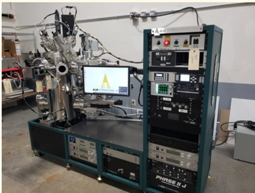
UHV AJA system in final factory checkout.
