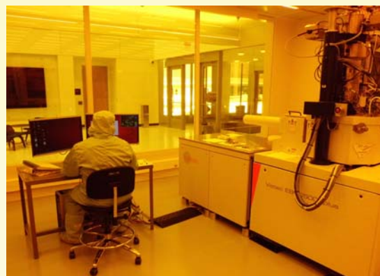
A user operating the Vistec e-beam lithography system. Notice the atrium and the main building entrance just outside the clean room.
