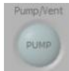
Fig 3. To Pump/Vent valve to evacuate chamber
