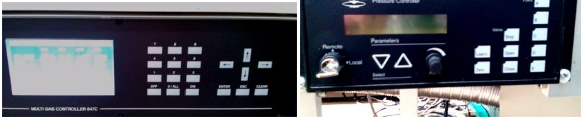
Fig3. 647 flow controller left and close up of the 651 pressure controller right image.
