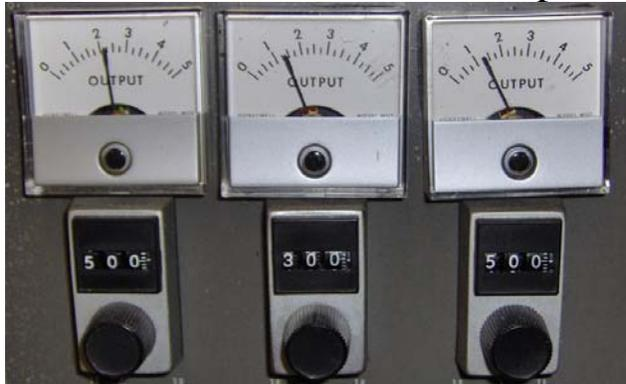
Fig. 6 Main temperature controls for the three zones.
