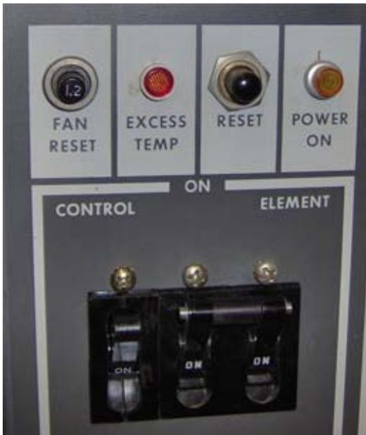
Fig. 4 Main power Control & Element switches.
