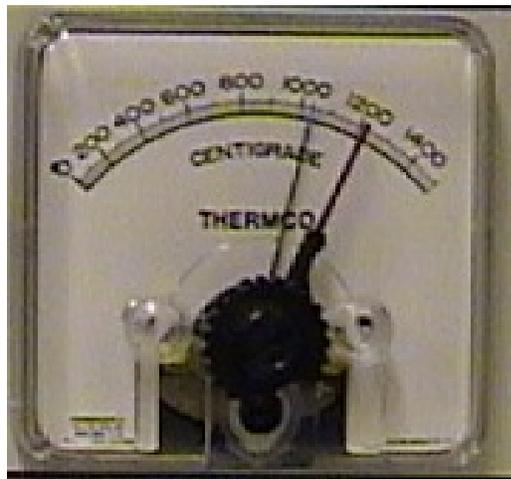
Fig. 5 Temperature readout display – black thin line
