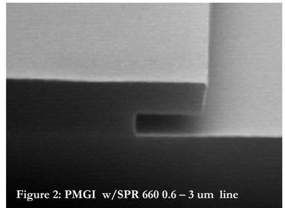
Figure 2: PMGI w/SPR 660 0.6 – 3  $\mu$ m line
