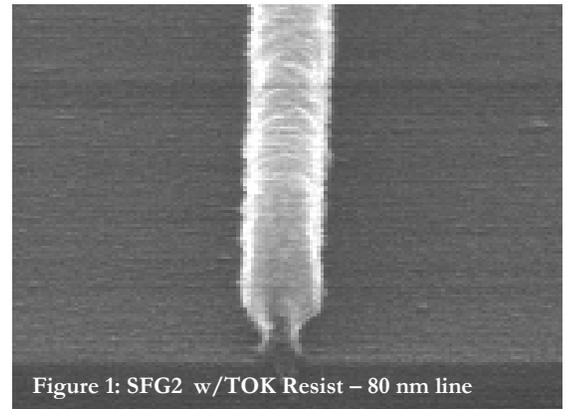
Figure 1: SFG2 w/TOK Resist – 80 nm line
