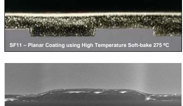
SF11 – Conformal Coating with Low Temperature Soft-bake < 190°C
