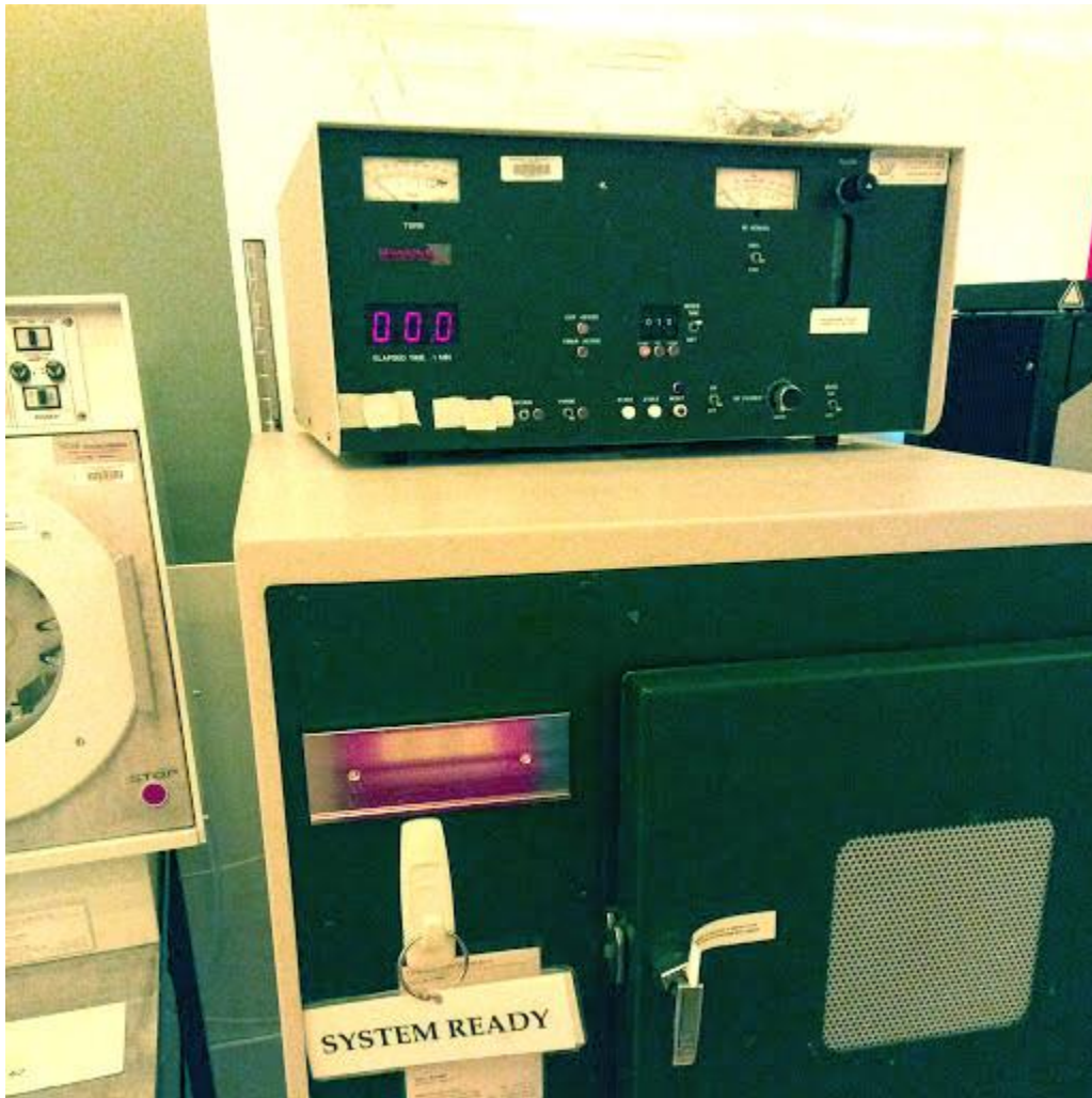
Figure 1 The oxygen asher, located in Keller Hall-Bay 2.
