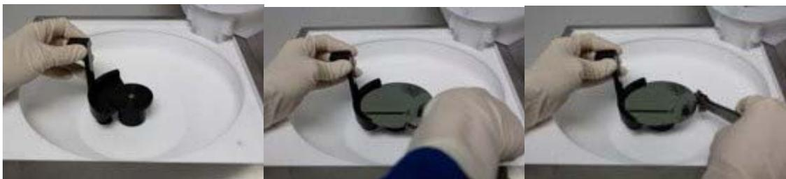
8. Press **Start Centering**: The spin chuck spins for the 5 seconds to test for centering. Centering can be restarted by pressing the Center button. *NB: Centering happens whether the lid is open or closed.*
