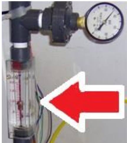
Fig. 2 Confirm the water is flowing before starting, the metal indicator should be in the middle of gauge.
