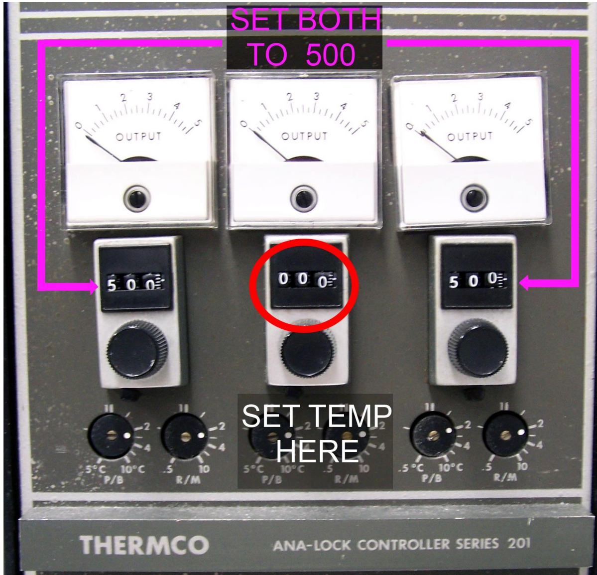
Fig. 6 Main temperature controls for the three adjustment knobs.
