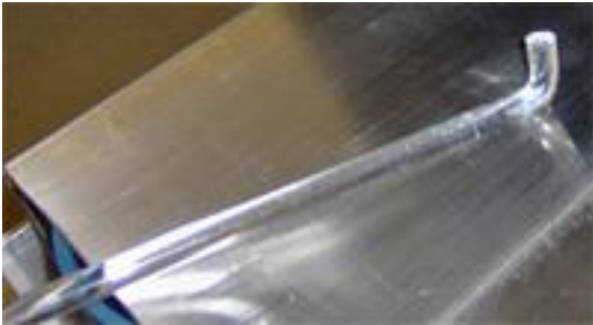
Fig. 4 Loading the samples should be done with this quartz rod. Do not handle the hook end, keep it clean.
