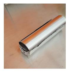
Figure 2 Use the boat former to mold the aluminum foil. The boat should not be longer than the boat
