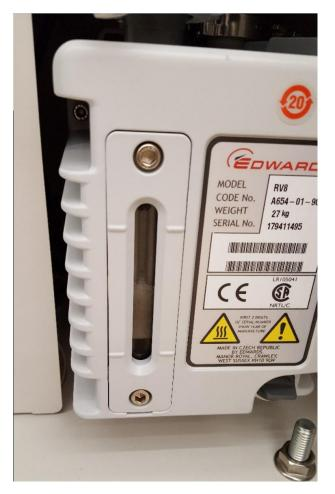
*Figure 9* Frothy oil in the pump is a telltale sign the pump is working too hard.
