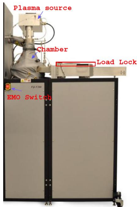
Fig 1. Main items of the Fiji ALD system.
