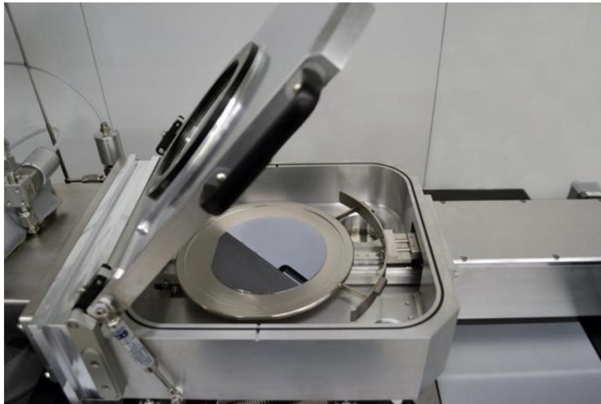
Fig 2. Vented load lock and wafer is in the correct position.
