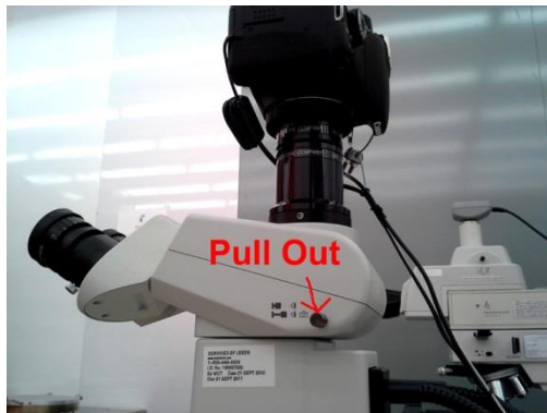
To make image viewable pull knob out.
